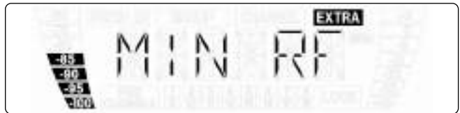
Example 2: Minimum RF level: -85 dB
