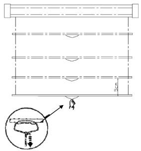
times to loosen up. If this happens, carefully with a little force yank the screen straight down to unlock the screen.
