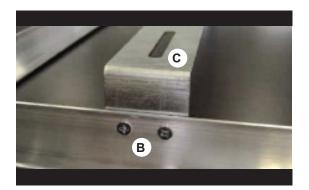
After that, mount the two iron brackets for the threaded rods using the proper holes that you find on the aluminium profile. (you will find the threaded rods inside the packaging of projector lift PPL 2035, PPL 2100 or PPL 2170)
