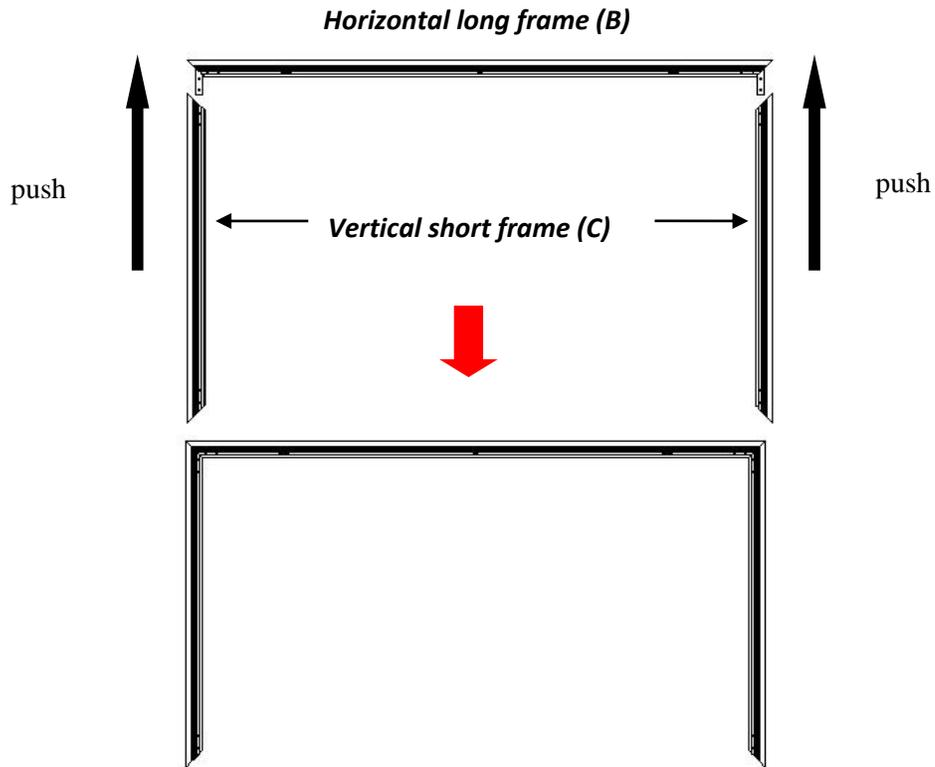
6. Join the remaining *horizontal long frame (B)* with the frame built in the previous steps as shown below.
