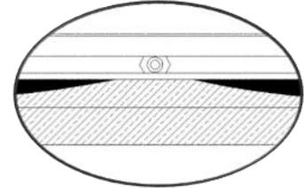
Lay the Velcro end on the screen material over the Velcro end of the frame and keep it within the edge.
