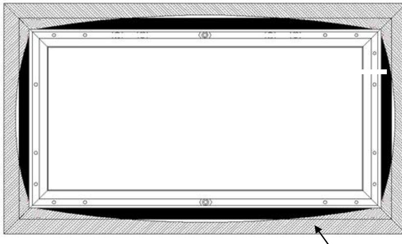
**Note:** The black shaded part represents the velcro on the frame. That Velcro end will ultimately attach with the other velcro end on the screen material.
