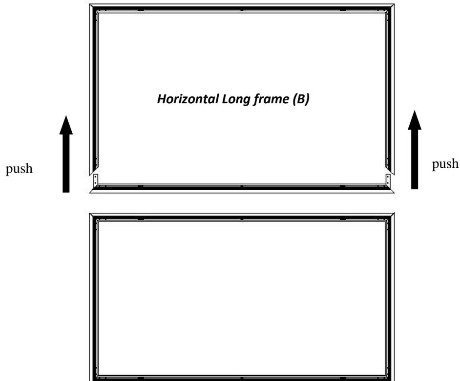
7. Make sure all four corners are properly in place to form a perfect square. Then fasten the four angles with the **M5x15 Screws (G)**.
