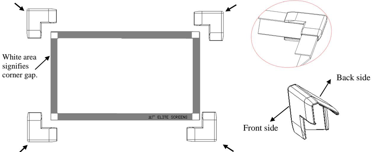
Once all corner sleeves have been snapped into each corner of the frame, it is ready to be installed.
