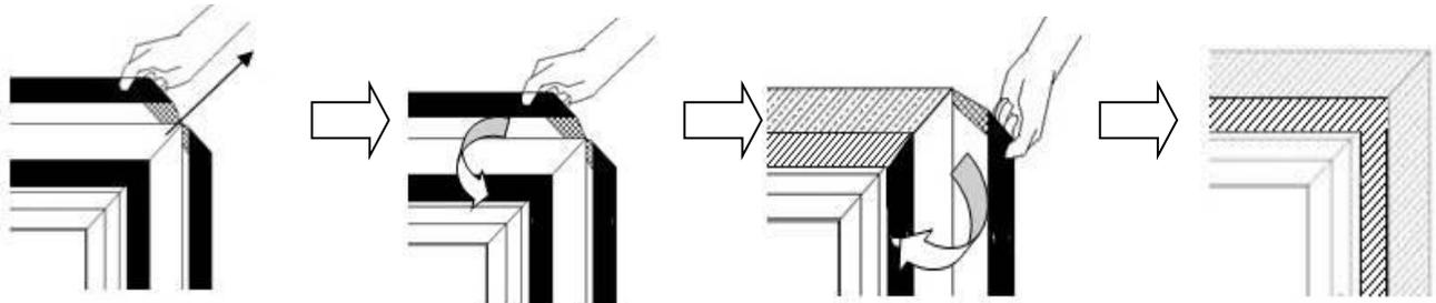
1) Stretch the screen material in the direction of the arrowhead.
